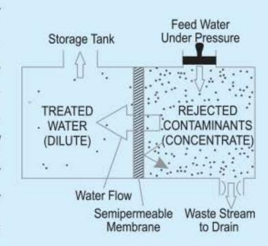
diluted end. Dissolved salts present in water as charged ions, get repelled by the RO membrane and are not allowed to pass through. Similarly, bacteria and germs are also blocked by the ultra fine pores of the RO membrane. These rejected impurities suspended on the concentrated end of the membrane are washed away in a stream of waste water, preventing the membrane from clogging.
